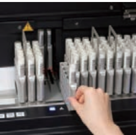
Set the tray on the rack sampler and start measurement.
