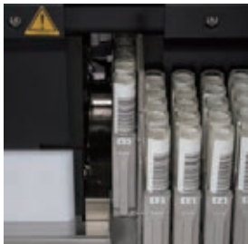
The rack at the left end is loaded into the analyzer, and the cup sensor recognizes the samples. The barcode reader then reads the sample IDs.
