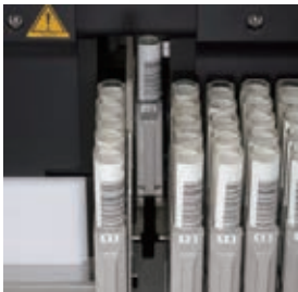
Racks for which sampling has been completed are pushed out of the analyzer and moved to the left end of the sampler.
