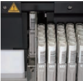
The rack is moved to the left and sampling is performed.
