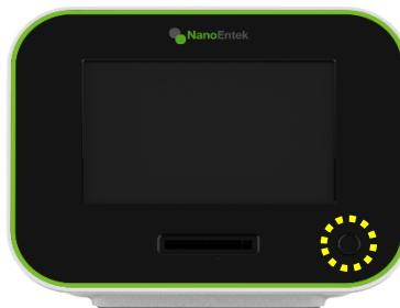
4. Press the power button for 3 seconds.
